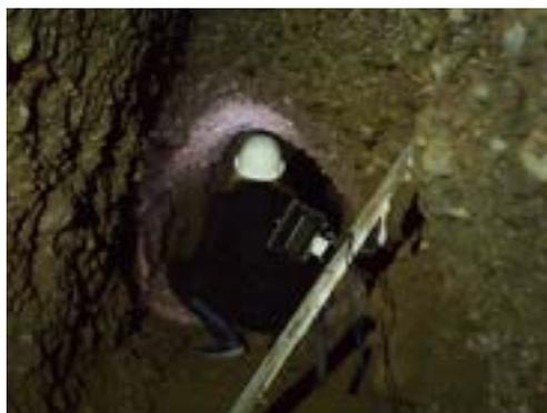
**Figure 4** – Two Hydrophones were placed in Ravne Hypogeum in Visoko (Bosnia-Herzegovina) for recording resonance in the ancient structure. There was almost 8-10cm of water on the bottom of the floor, so the Hydrophones were the most adapt device for recording vibrations in these conditions (Debertolis and Savolainen 2012).
