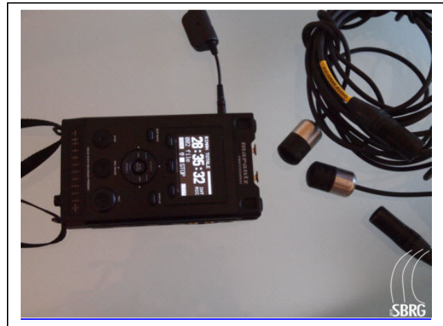
Figure 3. One of the digital recorders used (Marantz PMD661) and omnidirectional microphones which can be used under water (Hydrophones Aquarian H2a-XLR)
